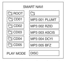
In stop mode, use ▲/▼, ◄/► on the remote control to select the item or folder (such as CD01, CD02...), and press **ENTER** button on the remote control to confirm, then select the desired track (such as 001 PLUMT, 002 RZID...) on the
